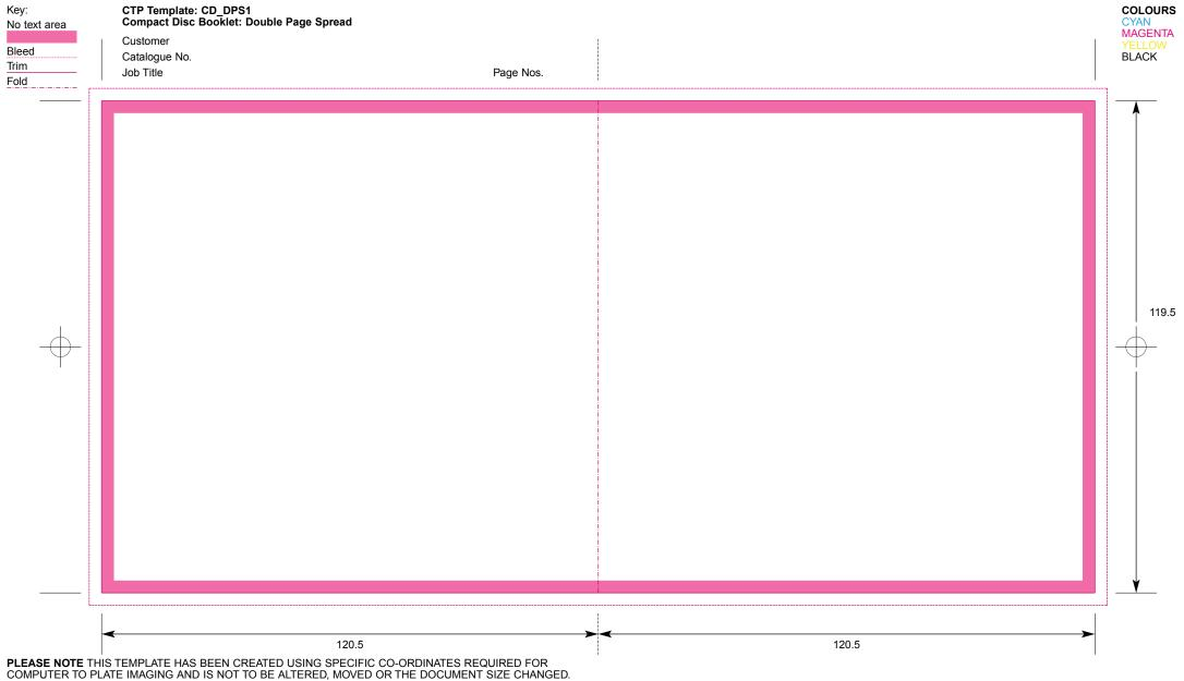
ALL DIMENSIONS ARE IN MILLIMETRES. BLEED ALLOWANCE OF 3MM ON TRIMMED EDGES
